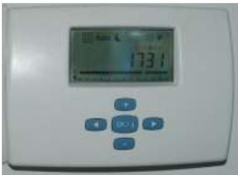
To set up the time use the arrow to move the box to the clock icon.
