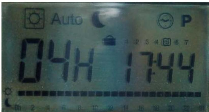
In this case the controller reverts to Automatic after 4 hours.
