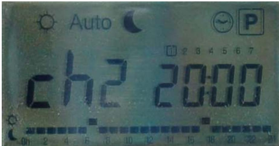
Select heat on with the **+** button, and heat off with the **-** button. You can backtrack and move forwards using the left and right arrows. All days should be completed, (When the little bars are raised, this means the heat is on for these hours).
