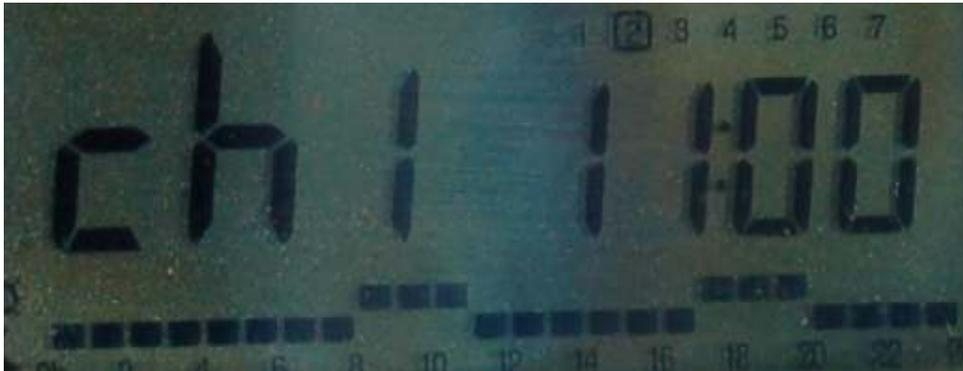
Select heat on with the **+** button, and heat off with the **-** button. You can backtrack and move forwards using the left and right arrows. All days should be completed, (When the little bars are raised, this means the heat is on for these hours).
